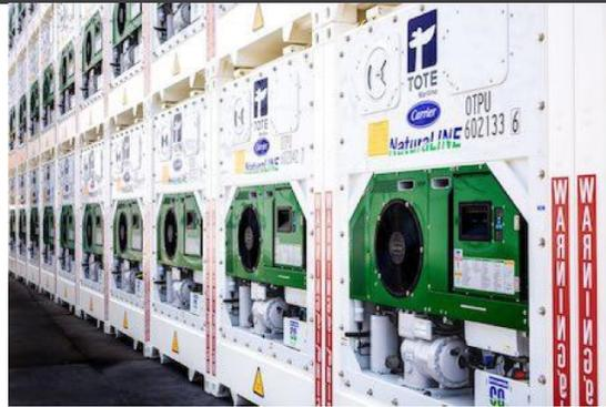
*TOTE Maritime Puerto Rico's latest investment in green technologies is the addition of 220 containers leased from SeaCube Containers and refrigerated by Carrier Transicold NaturalLINE units, which use the natural refrigerant carbon dioxide, with an ultra-low global warming potential.*
